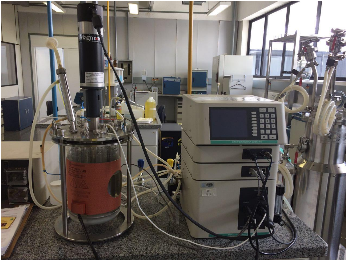
Figure 1. Autoclavable 3 L, BioFlo 110 bioreactor (New Brunswick Scientific).
